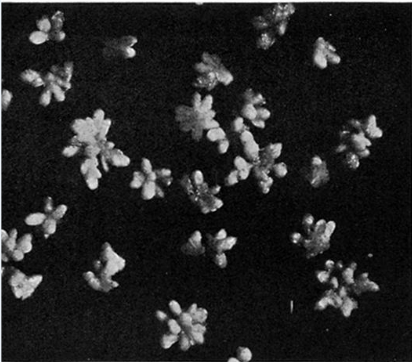
Fig. 10—Lead chloride, slow crystallization from 0.75% dextrine solution \times 10
