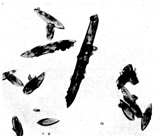
Fig. 8—Lead chloride, rapid crystallization at 25° from 0.25% dextrine solution \times 100
