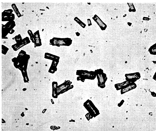
Fig. 19—Showing incipient spherulitic growth \times 250
