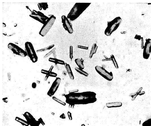
Fig. 17—Rapid crystallization from 0.5% dextrine solution at 50^\circ \times 200
