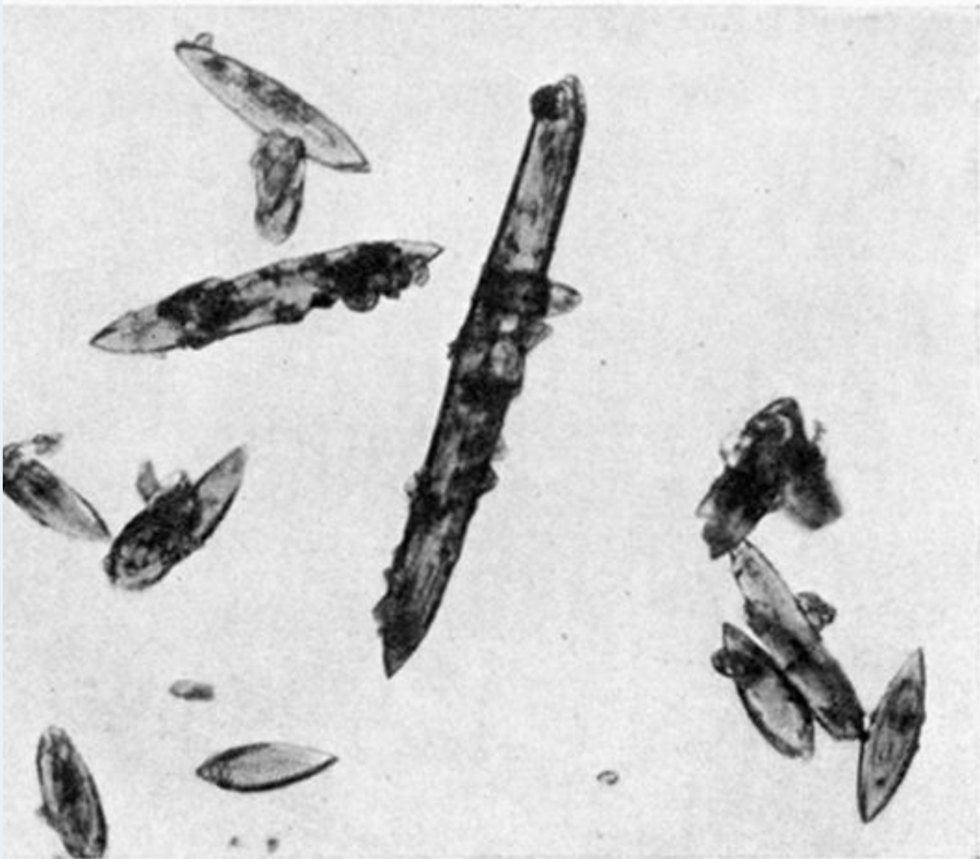
Fig. 8—Lead chloride, rapid crystallization at 25^{\circ} from 0.25% dextrine solution \times 100
