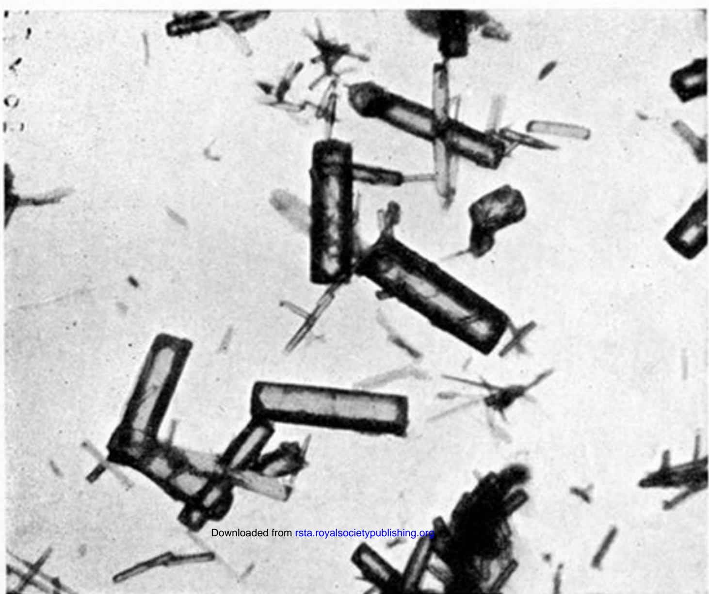
Fig. 16—Rapid crystallization from 0.25% dextrine solution at 80^\circ \times 200
